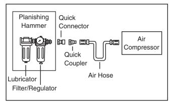
Figure 2. Correct air supply setup.
